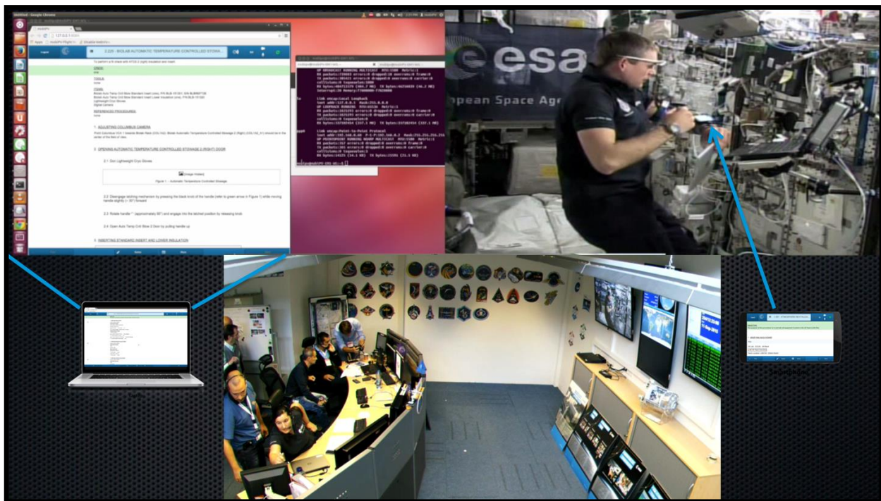
Figure 6. Live space to ground mobiPV operations. Ground terminal and ISS devices synchronized (ESA).
