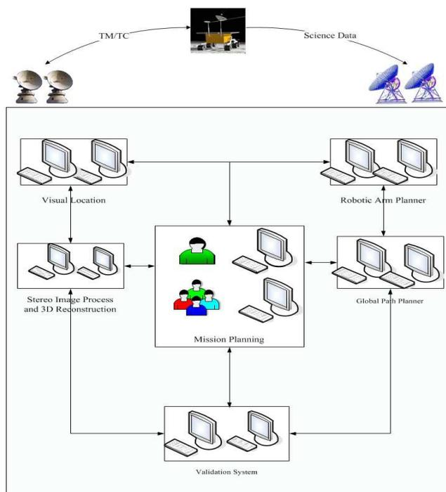
Fig 4 the overall architecture of the teleoperation system
