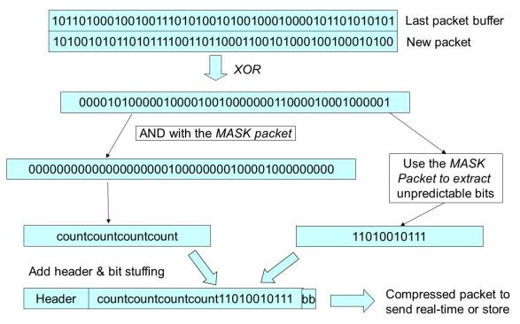
**Figure 1. The on-board element.** The diagram shows the operations that must be computed on-board to compress a single packet before it is streamed or stored. The "XOR" arrow implies points 5 and 6 of the previous numbered list, involving the initial XORing, inversion and horizontal correlation to produce the processed packet.
