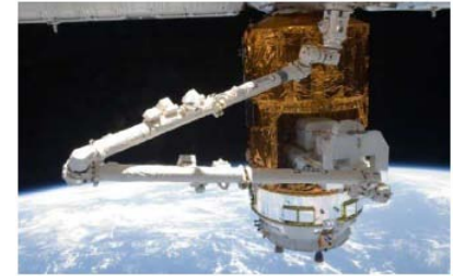
Transfer of the Exposed Pallet (EP)
