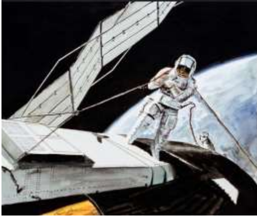
Fig. 3: Artist's concept of an EVA to free the solar array system wing. [4]
