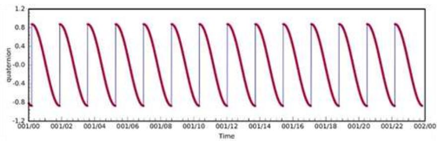
**Fig. 3 The data training output for the second components of the quaternions, which has 4 components. The red dots are the data values, and the blue lines are data training outputs. The neural network with two hidden layers is implemented for the quaternions.**
