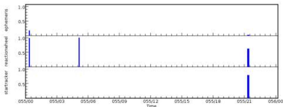
**Fig. 13 The event plot for NPP data on 2019/055. The around 21:16z shows that the relative strengths of DPCs are not dominated by the Star-Tracker or Reaction-Wheel subsystem, and there is also a small data pattern change in the Ephemeris Subsystem in the event.**
