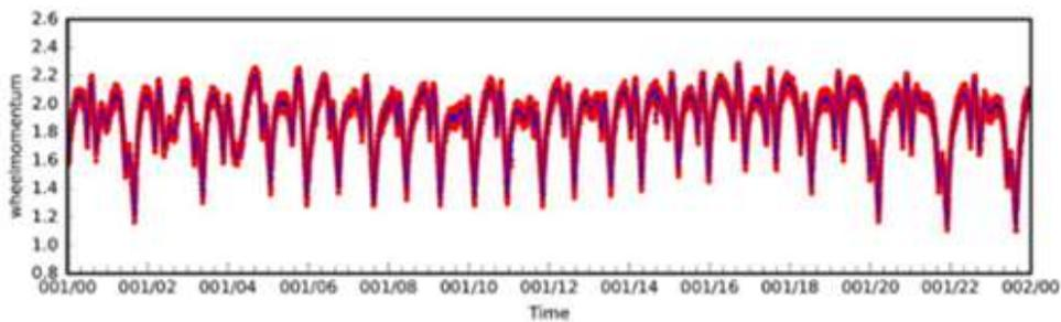
**Fig. 6 The wheel momentum in y direction, which is a linear combination of 4 relation wheel momentum. The red dots are data values, and blue lines are data training outputs.**
