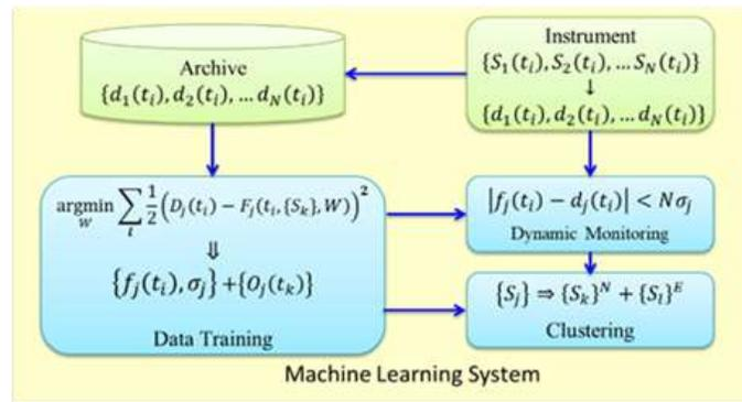
Fig. 1 The ML processes for satellite health and safety telemetry
