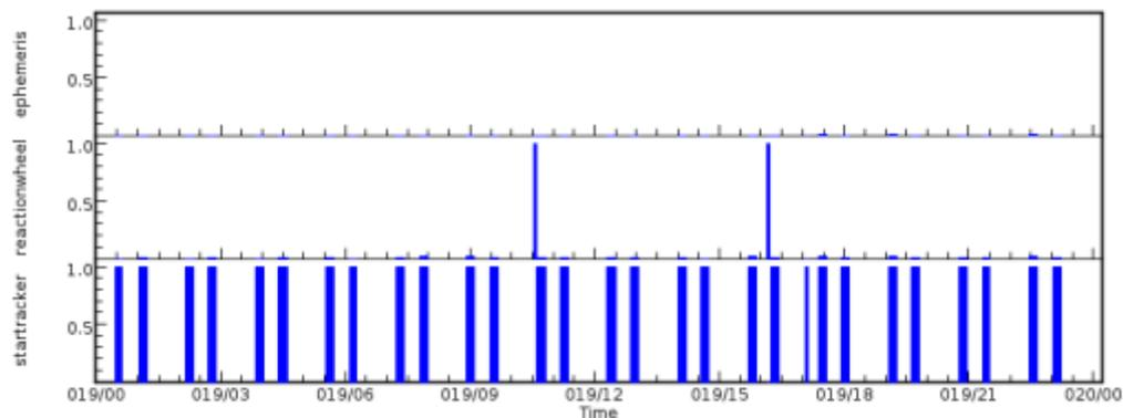
**Fig. 12 The event plot for NPP telemetry data on 2019/019. The events are mostly dominated by the DPCs in the Reaction-Wheel or the Star-Tracker subsystems. There are small contributions from DPCs in the Ephemeris subsystem.**
