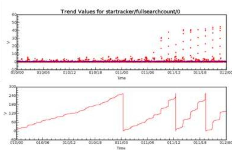
**Figure 7** The full search count in the Star-Tracker subsystem. The plot at bottom is the original data. The plot at the top is the processed data used in the data training. The blue line in the top plot is the mean value of the processed data.
