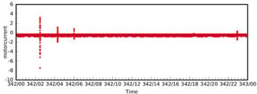
**Fig. 5 The motor current for the Reaction Wheel subsystem. The red dots are the actual data values, and the blue line is the mean value of the dataset in data training periods. The data points along vertical lines are treated as outliers representing DPCs.**
