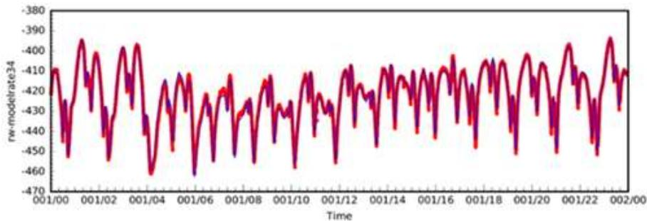
**Fig. 4 The momentum profile of the NPP reaction wheel 3. The red dots are data values, and the blue lines are data training outputs. The NPP satellite has a 4-reaction wheel configuration.**
