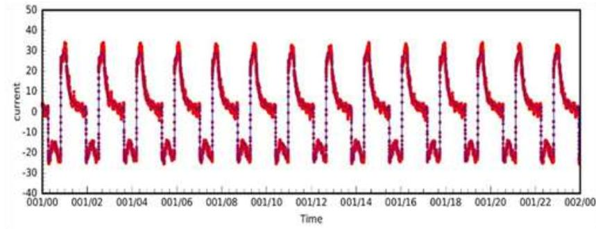
**Fig 2 Battery current of the NPP power system. The red dots are the data values and blue lines are data training outputs. The neural network with two hidden layers is implemented for this dataset.**
