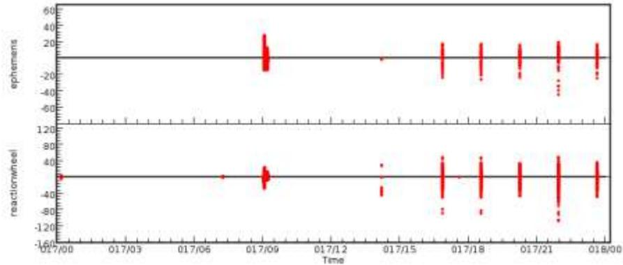
**Fig. 8** The outlier plot at the subsystem level for the reaction-wheel (bottom) and ephemeris (top) subsystems of NPP satellite. The outliers at the subsystem level include the outliers of all datasets in corresponding subsystem. Values of outliers are determined by Eq. 8.
