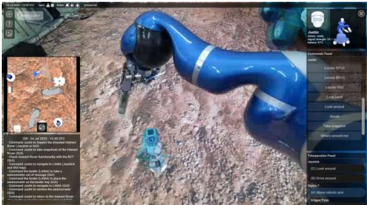
Fig.2 The Surface Avatar experiments make it possible for NASA astronaut Frank Rubio to see the world through the eyes of a robot. The image shows the perspective of the humanoid DLR robot Rollin' Justin as it places a seismometer on the ground. For orientation in space, there is a small map on the left side of the image. On the right side are the command options that the robot can receive from the astronaut, which include the commands for scaling the autonomy of the robot. (Credit DLR ©. All rights reserved)
