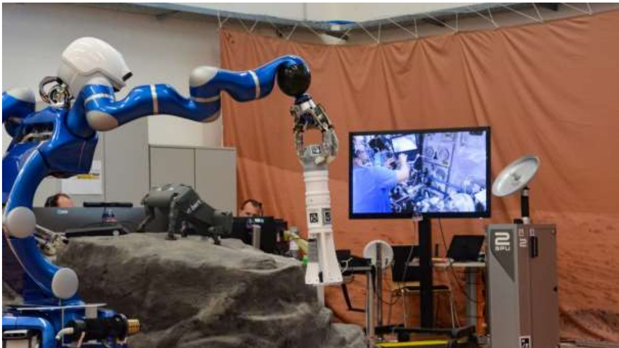
Fig. 1 NASA astronaut Frank Rubio operated the robot team located at the Mars laboratory from onboard the ISS. As part the first Surface Avatar experiments, humans and robots were tasked with retrieving a scientific instrument – in this case a seismometer – from the lander and placing it in the mission area. (Credit DLR ©. All rights reserved)
