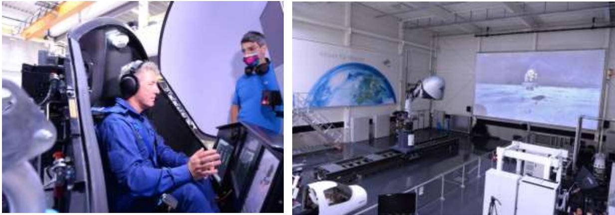
*Vittori inside the simulator capsule (nose cone open), on the right the closed nose cone and the panoramic view of the landing site as presented to “mission control” during Vittori’s touch down of his simulated lunar landing vehicle.*
