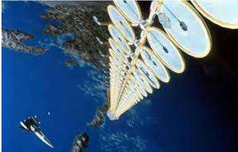
The SunTower SPS concept, assumed 1000W/kg of specific power, while the thin-film based European Sail Tower SPS concept assumed 3500W/kg global specific power (including sail deployment mechanism, 4850W/kg if only taking the sail into account) with 13% efficiency CIS deposited on 7.5 $\mu$ m thick Kapton® foils. [3]
