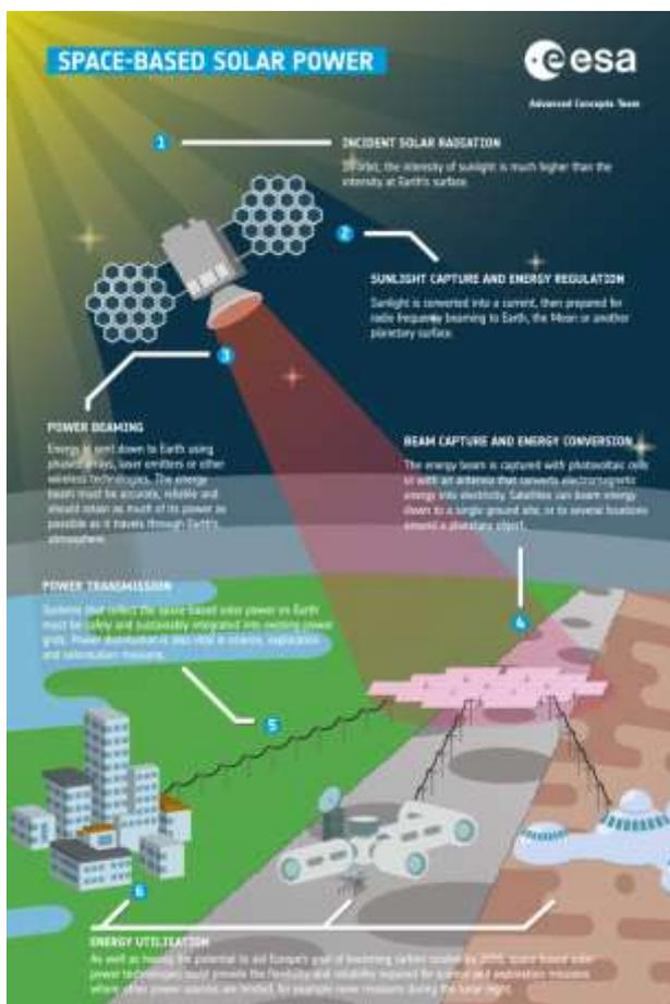
For satellites orbiting high above Earth, outside the atmosphere, sunlight is on average more than 10 times more intense than on the ground in Europe. SBSP satellites could also face the Sun all day every day to continuously capture the maximum amount of light possible. The satellites could then beam energy down to Earth, the Moon or other planets.
