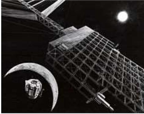
Artist's concept of a solar power satellite in place. Shown is the assembly of a microwave transmission antenna on the left. The solar power satellite was to be located in a geosynchronous orbit, 35,786 kilometers (22,236 mi) above the Earth's surface (NASA 1976). [2]
