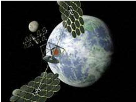
SERT Integrated Symmetrical Concentrator SPS concept (NASA), consisting of two symmetrical ultra lightweight arrays of "SolarSailType" solar concentrator mirrors in a space-frame structure (symmetrical mirror arrays shown on-top and bottom of the image).
