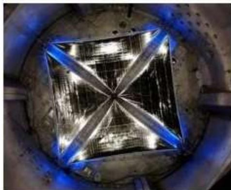
Vacuum deployment of a 20m x 20m solar sail made of CP1TM polyimide and CFRP masts in the NASA 30m Plum Brook Facility (courtesy of NASA, SRS, ATK-Ab). [3]
