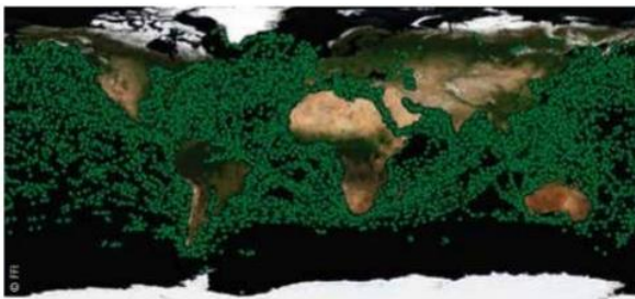
Fig. 1: ColAIS sample from June 1, 2010: From 19:00 to 9:00, the NORAIS receiver collected more than 90,000 Class A ColAIS messages.
