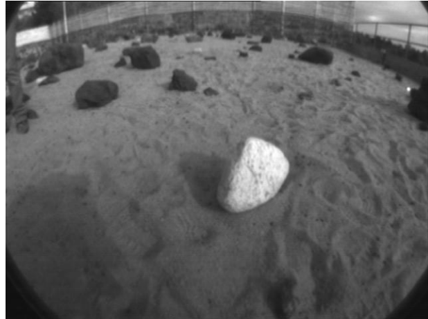
Figure 2. Image taken in response to a science alert on the JPL FIDO rover. In this test, science alerts were generated for “high albedo” (or light-colored) rocks.
